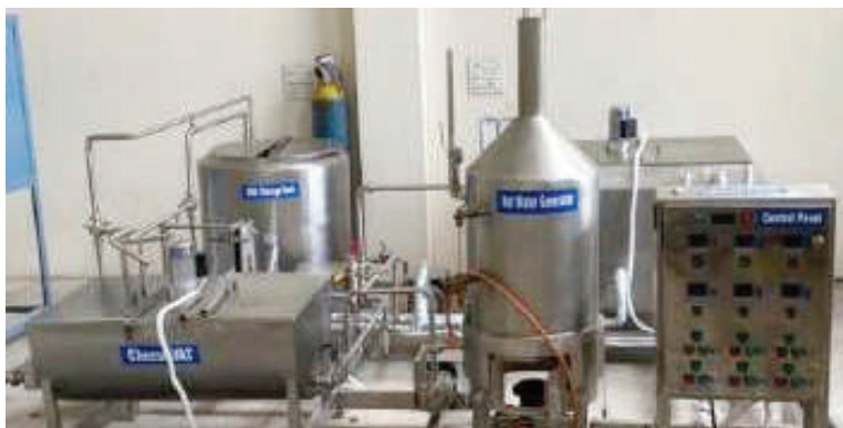
Fig: Mechanization of Mozzarella cheese manufacture machine
