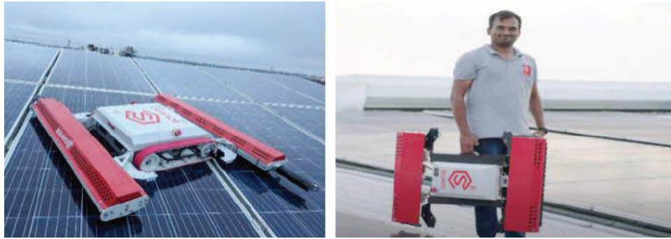
Fig.: Autonomous Solar PV Panel Cleaning Robot.
