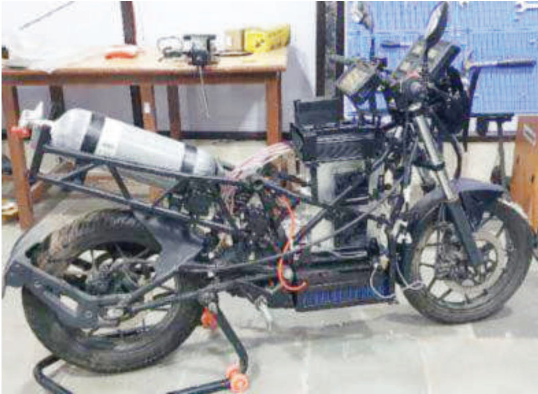
Fig.: Hydrogen fuel cell powered two-wheeler built by Hydrovert Energy
