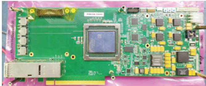
Fig.: Trinetra interconnect board
