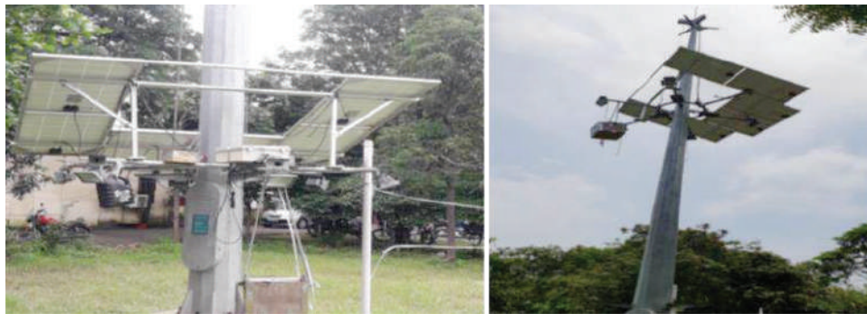
Fig.: Saur Stambh –for agri-iot applications.
