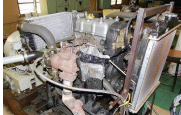
Fig.: Biogas engine test beds with subsystems
