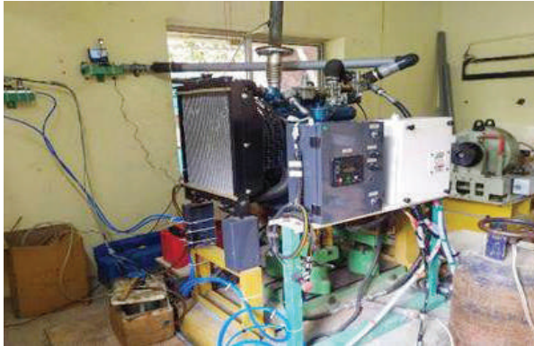
Fig.: Biogas engine test beds with subsystems
