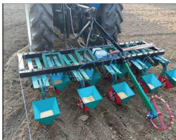
Fig.: Sensor-based precision seeding retrofit module for cultivators
