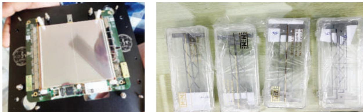
Fig.: Outer Tracker silicon module and mechanical components.
