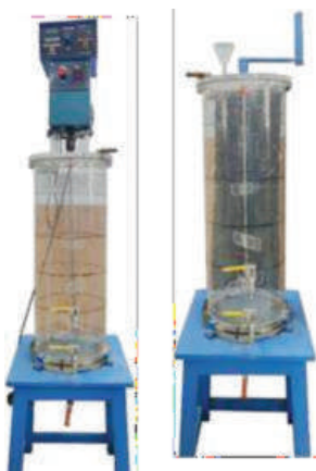
Fig.: coagulation-based domestic defluoridation kit
