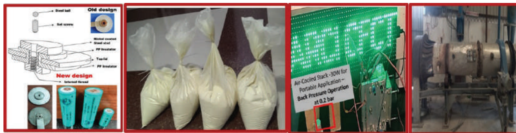
Fig. Development of lid assembly for Li-ion cell, large scale milled LFP cathode material, PEMF C (30 W) using air cooled and open cathode, and rotary calciner for the bonded magnets
