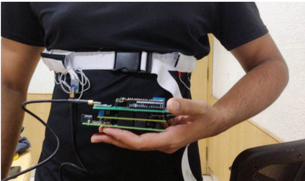
Fig. Wearable Bioelectrical Impedance Analyzer
