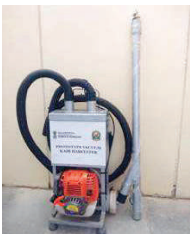
Fig.: Vacuum operated Kair harvester
