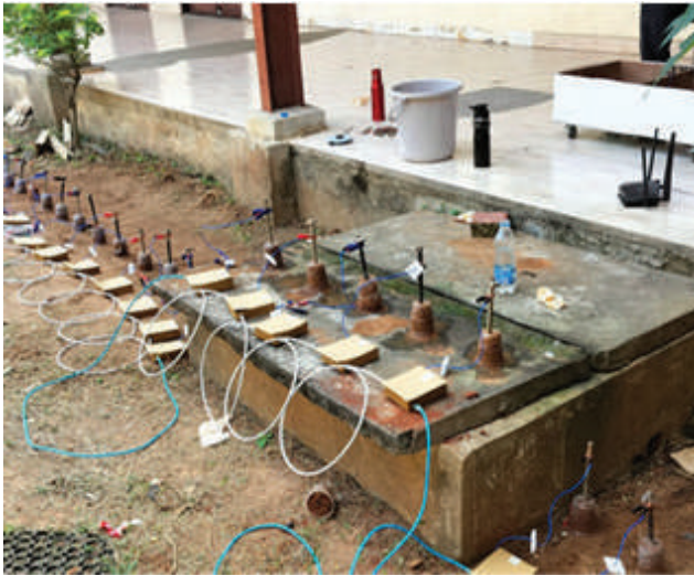
Fig. Sensing system for detecting underground hidden leak
