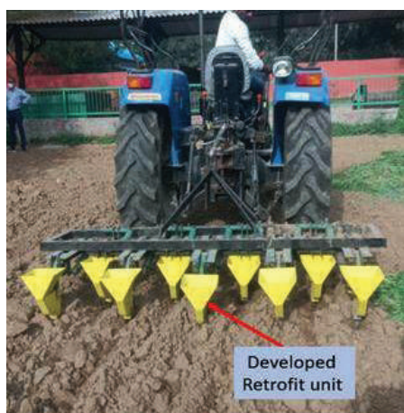
Fig.: Sensor-based precision seeding retrofit module for cultivators
