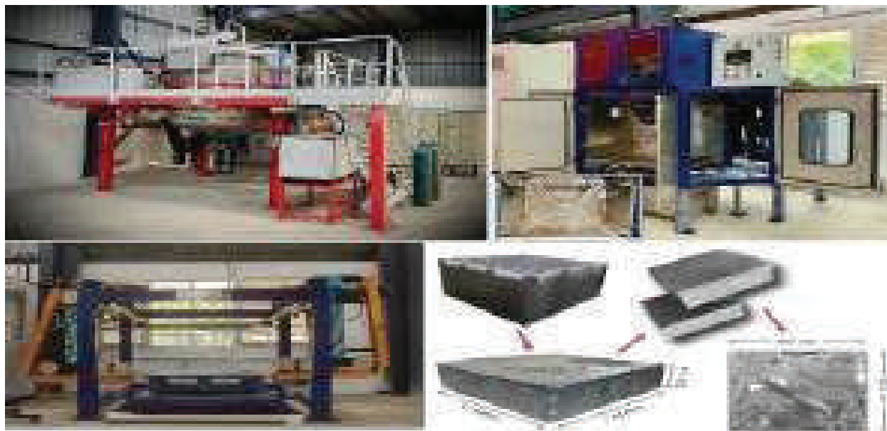
Fig.: 800kg multi-crystalline silicon solidification furnace and slicing machines.
