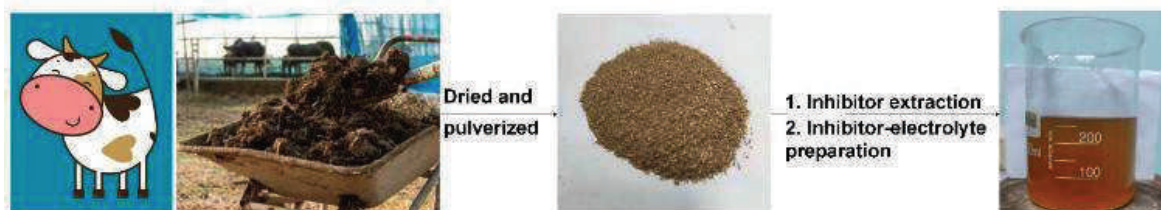
Figure 2: Flow of the processes followed to prepare the inhibitor-electrolyte solution.
