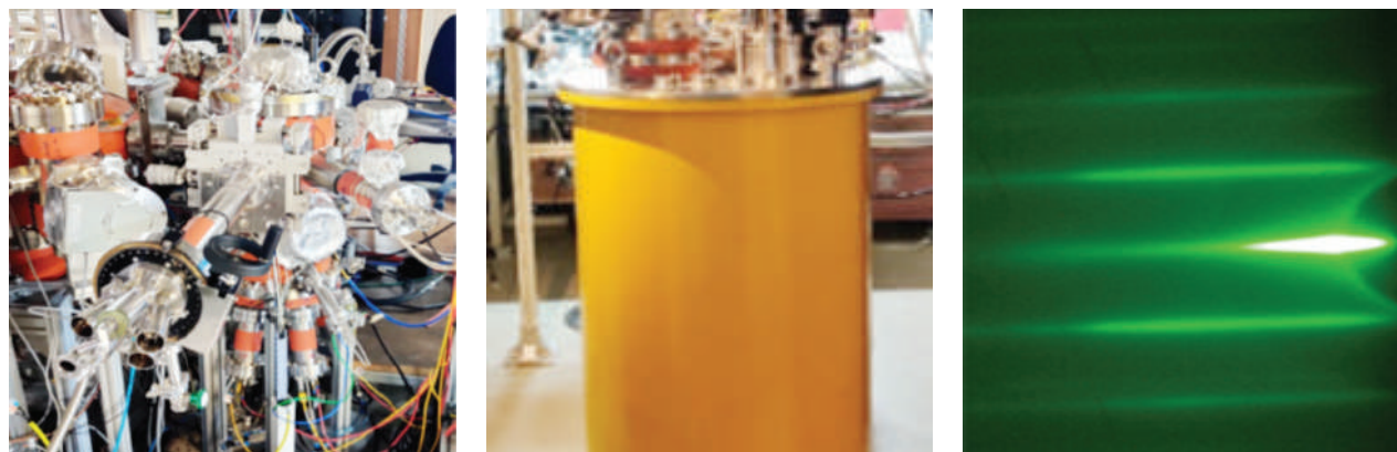
Fig.: In-house assembled Molecular Beam Epitaxy, VTI Cryostat, and RHEED output.
