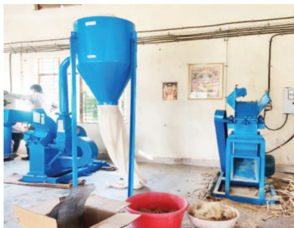
Fig.: Biomass-based pellet production unit
