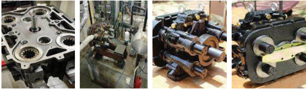
Fig.: Volumetrically Controlled Wankel Steam Expander for use with Low-pressure Solar and Process Steam.
