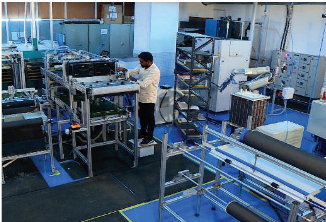
Fig. Automated PEMFC Components Stack Fabrication Pilot Line
