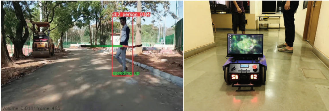
(a) Identification of pedestrians from monocular camera images (b) YATI, the robot used for experiments
