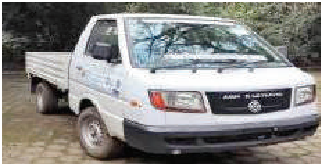
Fig.: Neat Methanol Hot Surface Ignition Common Rail Engine Demonstration Vehicle.
